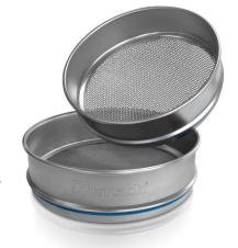
RETSCH test sieves are available in many sizes and varieties, primarily in the four frame sizes most widely used in laboratory analytics: 200 x 50 mm, 200 x 25 mm8"x 2" (203 x 50 mm), 8"x 1" (203 x 25 mm)
